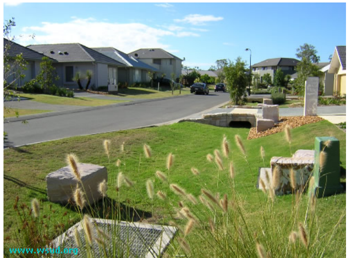
Figure 6: Examples of grassed swale (Source: Water Sensitive Urban Design of the Sydney Region)
