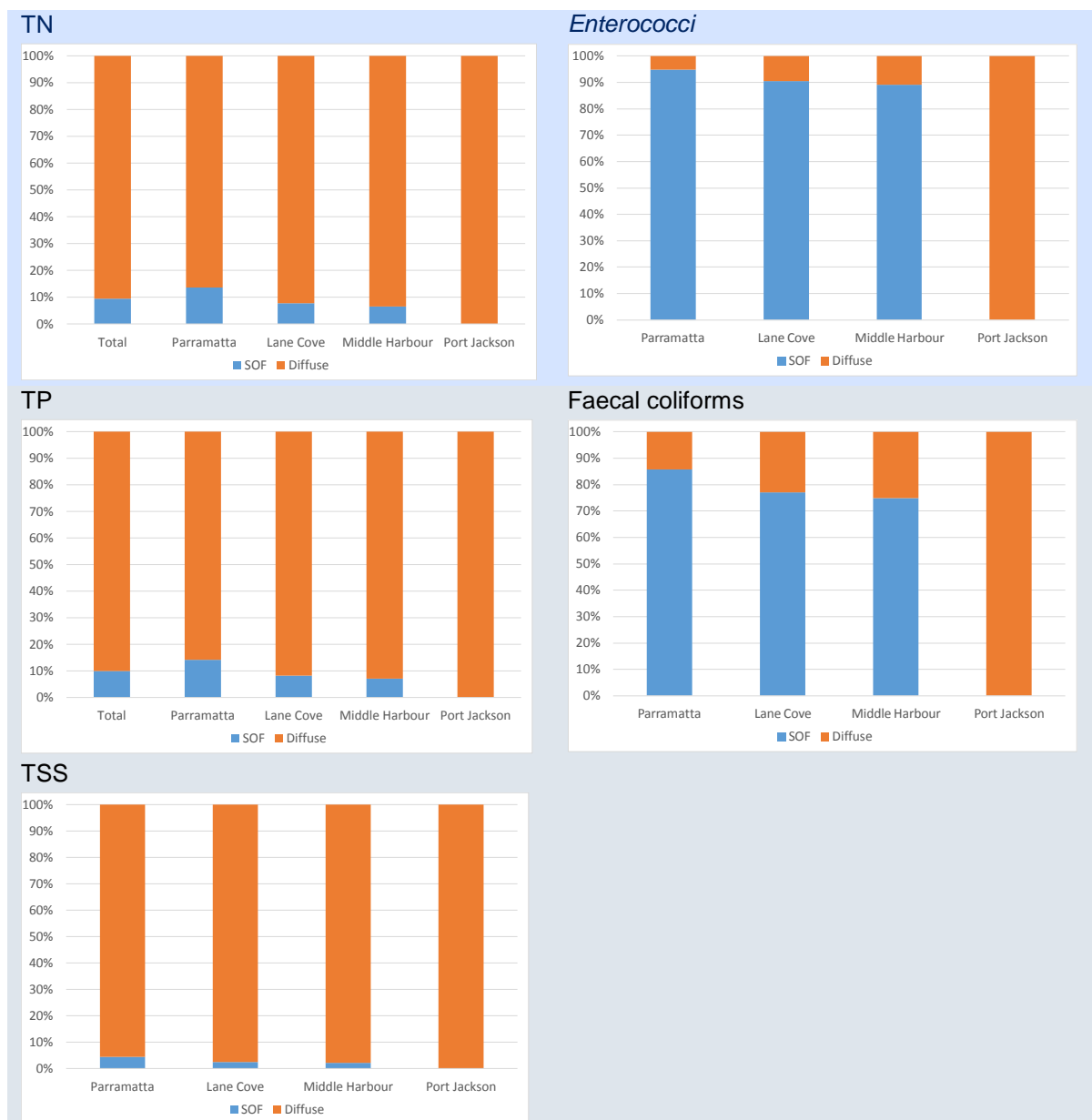
FIGURE 5. THE PROPORTION OF POLLUTANTS THAT IS CONTRIBUTED FROM SEWER OVERFLOWS (SOF) VERSUS DIFFUSE SOURCES FOR THE FOUR MAJOR SUBCATCHMENTS IN THE SYDNEY HARBOUR CATCHMENT
