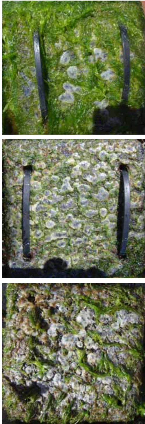
Figure 13. Replicates of W4 coated tiles from Malabar (top), Clovelly (centre) and Rozelle (bottom) showing accumulation of algae around wax treated areas.
