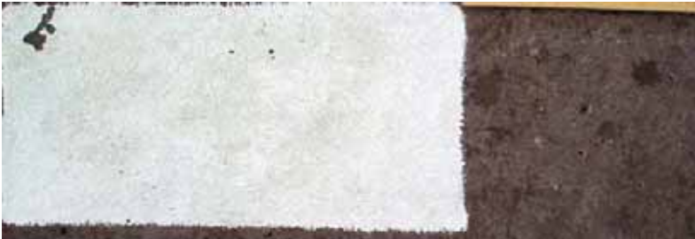
Photo 29 – Clovelly Bay Promenade Other X2 squares and adjacent control square. Note that it is difficult to assess presence of micro-fouling in control squares due to background colour of concrete
