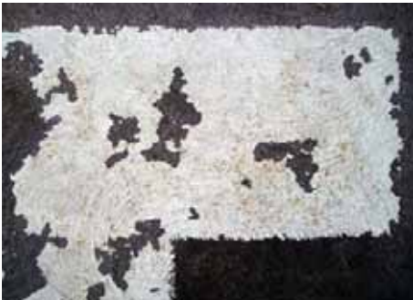
Photo 28 – Clovelly Bay Promenade X2 squares showing micro-fouling at 13 weeks and peeling of X2 paint
