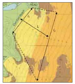
Figure 4.2 (reproduced from main report) Definition of parameters to calculate beach volume requirements
