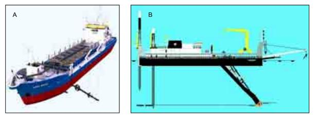
Figure 5.2 (A) Trailing Suction Hopper Dredger and (B) Cutter Suction Dredger
