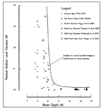
Figure 4.9 Measured Beach and Near-shore Seabed Fluctuations (Nielsen 1994)
