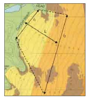
Figure 4.2 Definition of parameters to calculate beach volume requirements
