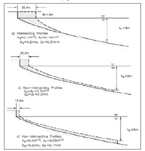
of the borrow material will affect the cross-shore shape of the nourished beach profile, sand loss rates and how the beach will respond to storms. This is demonstrated in Figure 4.7. The borrow sand compatibility is critical to the success of the nourishment campaign.
