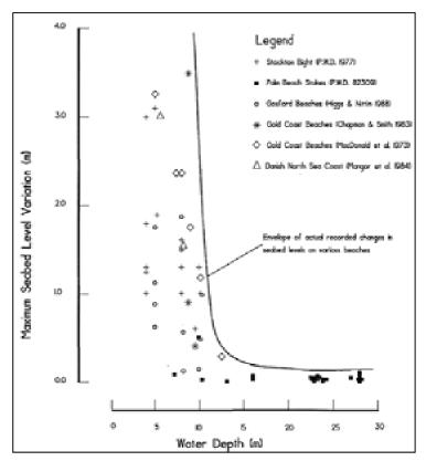
Figure 6.4 Measured Beach and Near-shore Seabed Fluctuations (Nielsen 1994)
