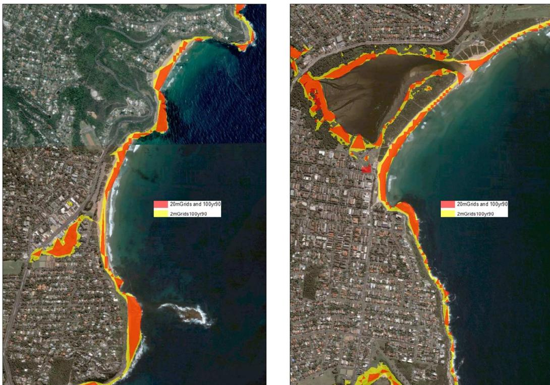
**Figure 35:** Examples of the areas of inundation based on the 1-in-100 year storm with 90 cm sea-level rise simulation overlaid on aerial photography. The adjacent elevation values from the LiDAR data that are below the corresponding water level have been calculated on the basis of LiDAR data at 2 m (yellow shading) and LiDAR elevations degraded to 20 m resolution (red shading).
