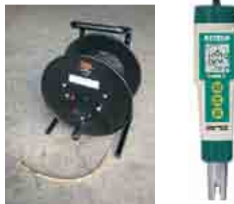
Figure 4 – Example of water level dipper and pocket sized salinity EC meter.
