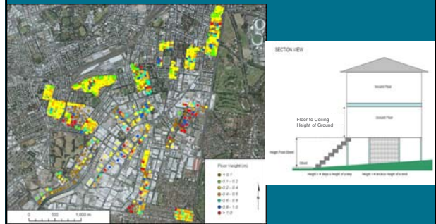
Map of distribution of building floor heights assessed by FIDAT (Maqsood et al., 2012)
