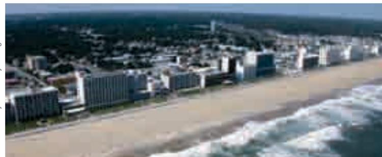
An estimated \$105 million in damage was prevented after Hurricane Isabel struck a nourished beach with a seawall at Virginia Beach in fall 2003. The project was designed to stop a 9-foot storm surge – and it did. The nourished beach minimized wave attack and overtopping of the seawall, the community's last line of defense.
