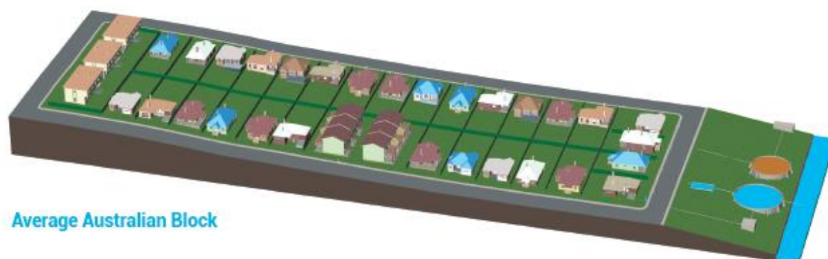
Figure 40: The contaminated stormwater (brown) is collected, stored and treated separately from the clean runoff (blue) (Dixon, 2015)
