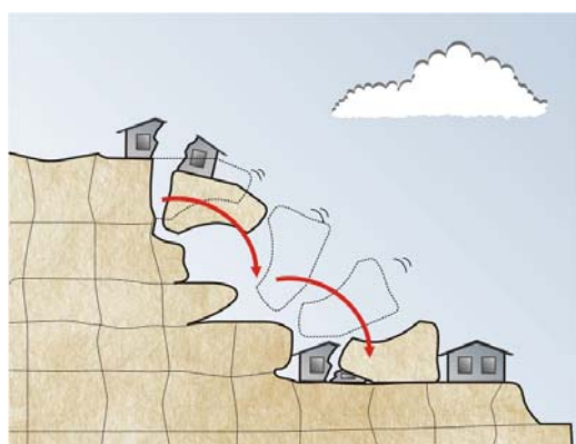
Figure 1 - Failure of an undercut block
