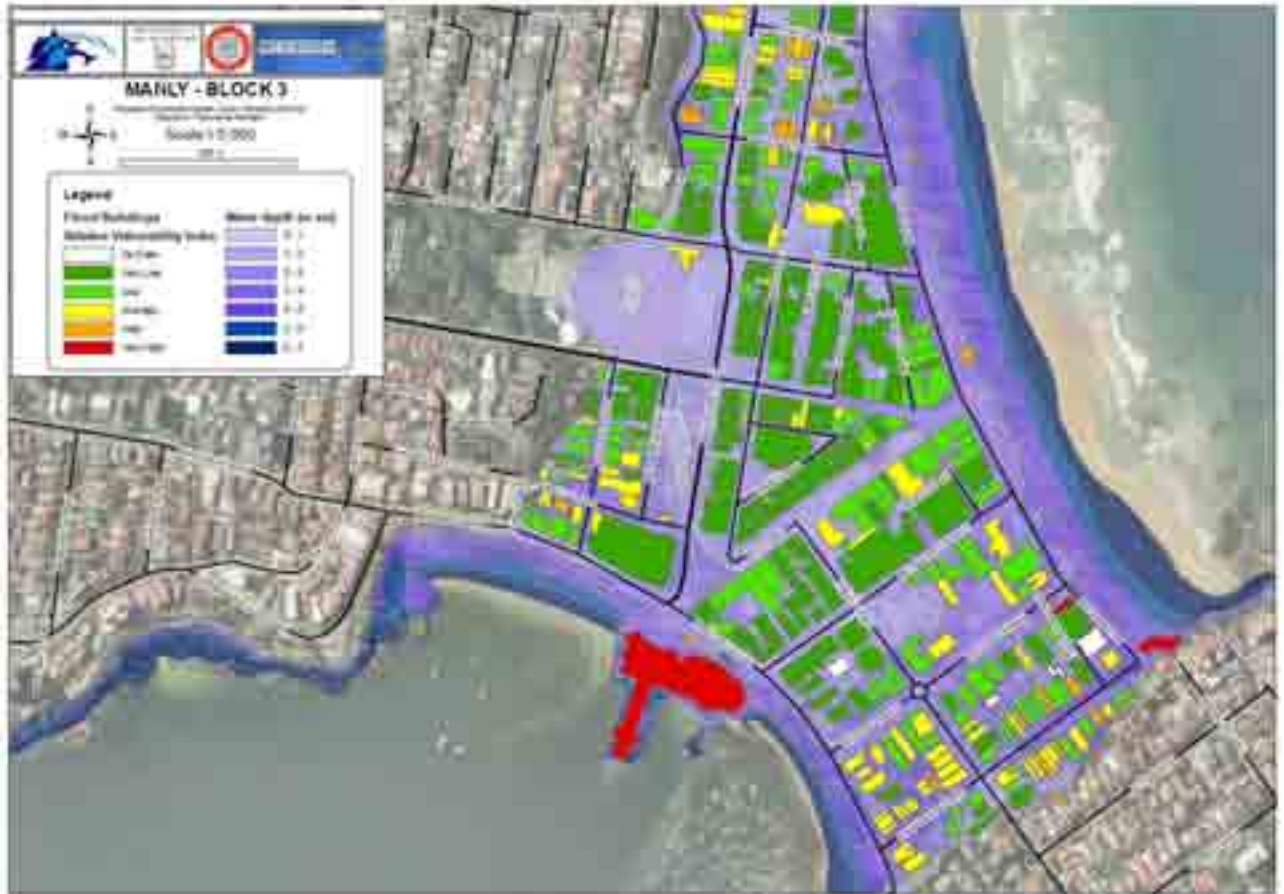
Figure 42. Tsunami inundation and RVI scores in Block 3, Manly
