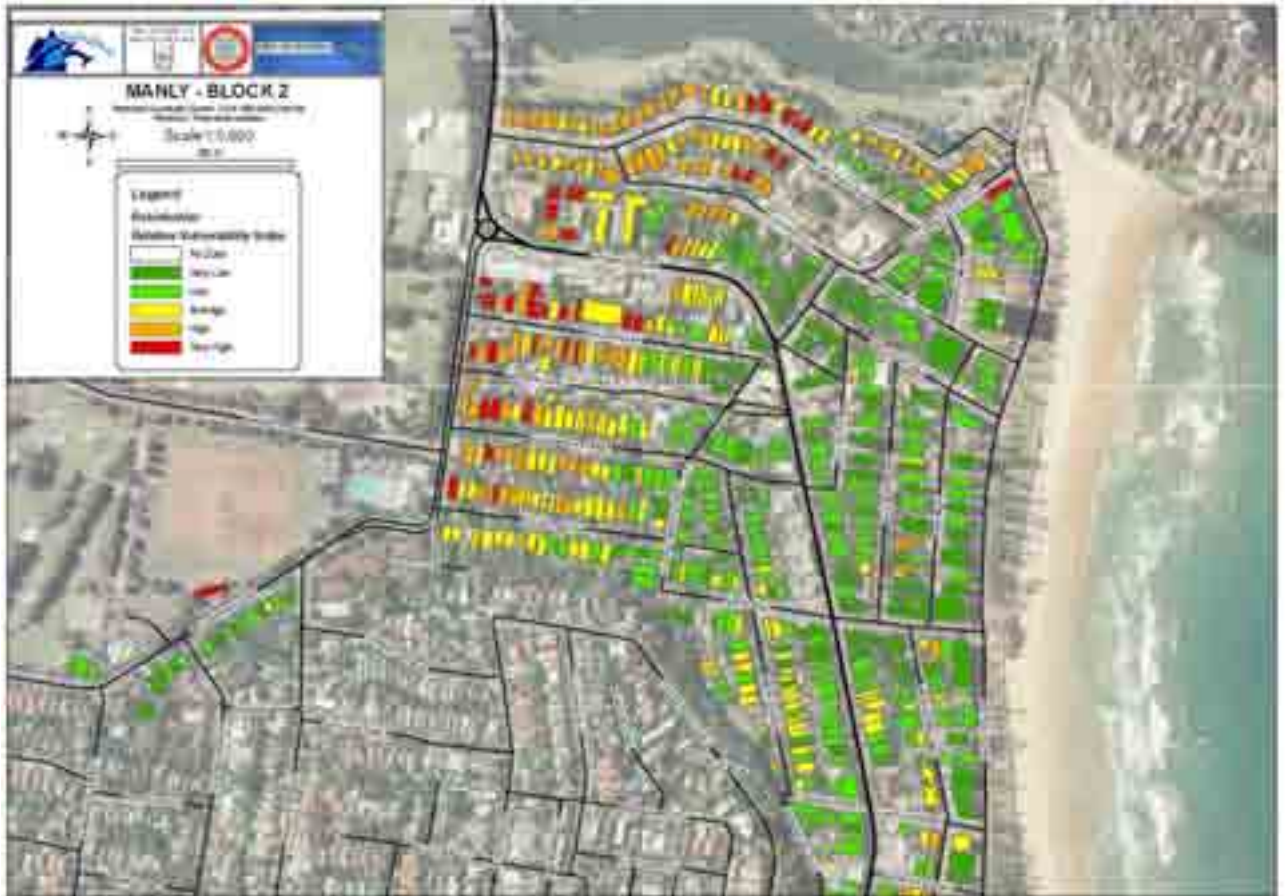
Figure 41. The RVI scores of residential buildings in Block 2, Manly
