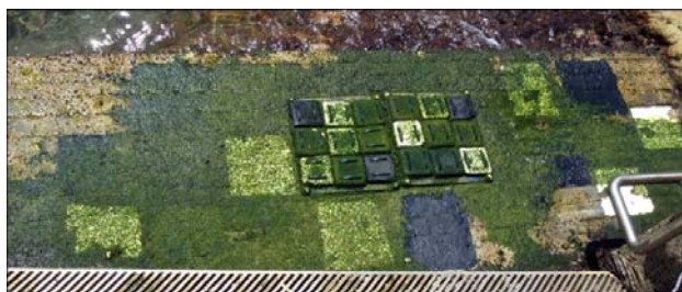
Photo 3 – Clovelly Step after 8 weeks. Most black-Y3 squares are heavily fouled (>75% cover) however two squares show less than 5% fouling cover. Most white-X8 squares are completely fouled but fouling cover is less dense than fouling cover on control (green/concrete) squares. Control squares are the same as at 5 weeks.
