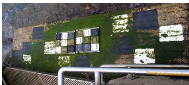
Photo 2 – Clovelly Step after 4 weeks. Black-Y3 squares showed 5–25% fouling cover while white-X8 (remaining white) squares showed 10–60% fouling cover. Most control squares (four of six) showed 100% fouling cover (now green) but two control squares had less than 10% fouling cover (Table B.1, B.2 for statistical analysis) Note: the tile experiment was added to the centre of this step after 1 week as white-X7 and blue-Z3 coatings painted here had peeled off by this time.
