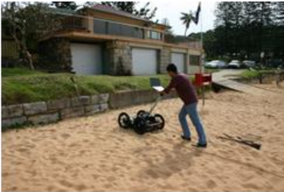
Figure 6 Collecting GPS and GPR data
