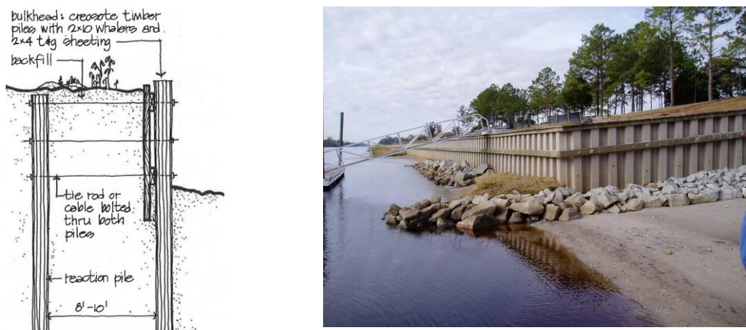
Figure 1 Illustration for Anchored Bulkhead Walls
