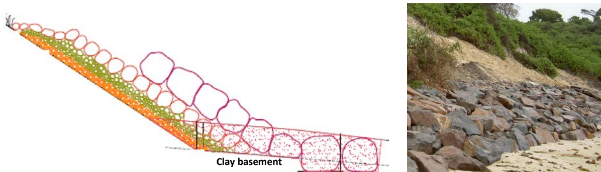
Figure 11 Rock rubble revetment
