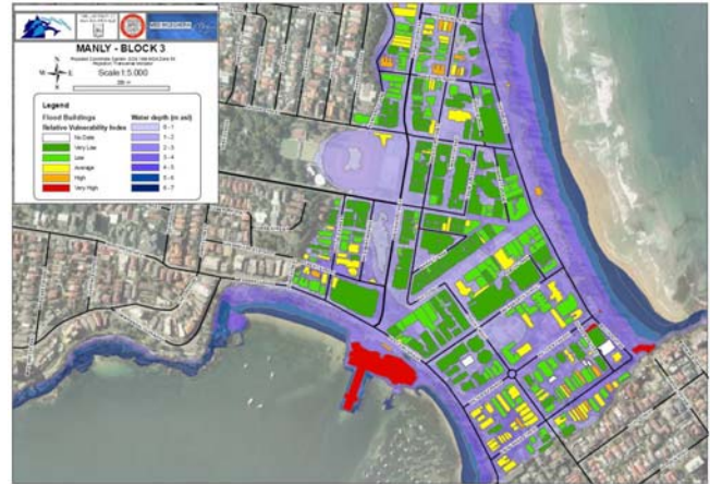
RVI scores of inundated buildings in Manly
